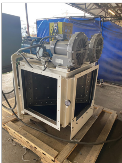
FIGURE 4. A flow-reversal indexing valve provides a zero-leakage design that utilizes a high-pressure air seal
