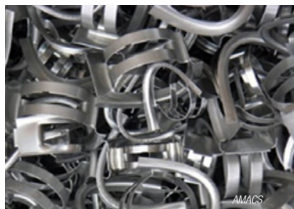
FIGURE 1. Amacs' fourth-generation high-performance Superblend ABS packing is a combination of various packing sizes, which provides the efficiency of the smaller and the capacity of the larger packing to provide enhanced benefits
