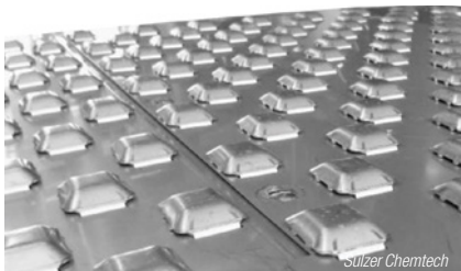
FIGURE 2. Sulzer's UFM valve trays were designed using computational fluid dynamics to ensure mixing between the vapor and liquid on the tray deck in order to maximize efficiency while simultaneously increasing capacity
